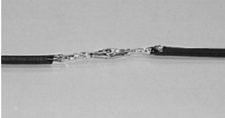
Center Heat Shrink Tube Over Cable
