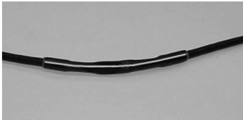
Center Heat Shrink Tube Over Cable
