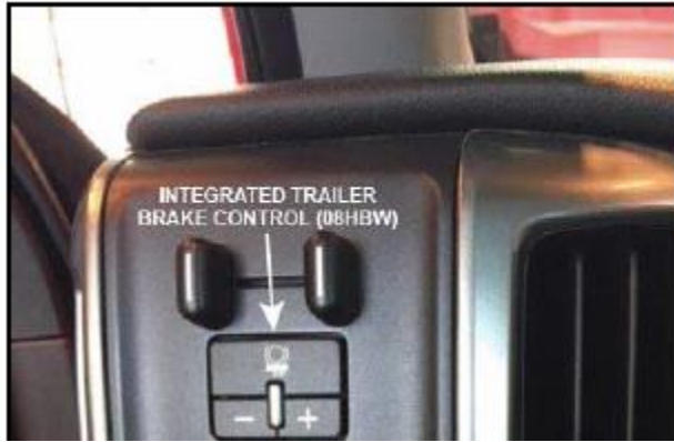
Figure 7.4.2.1: Integrated Trailer Brake Control Schematic
