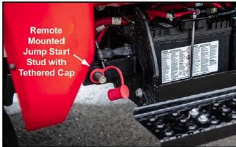
Figure 8.3.2: Remote Jump Start Stud schematic
