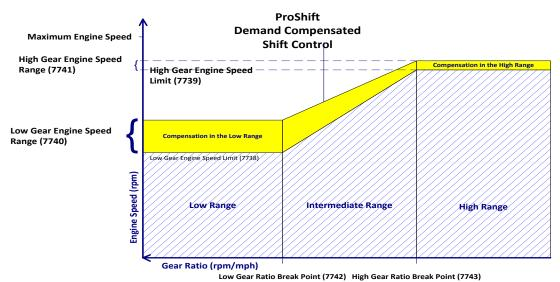
Progressive Shift consists of 3 gear regions: a high gear region, a low gear region, and an intermediate region. The gear ratio break point parameter settings determine what range the gears fall within.
