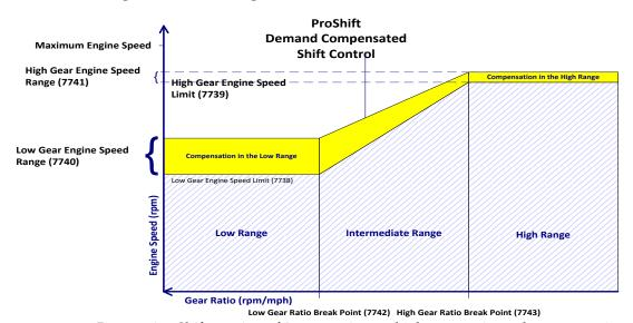
Progressive Shift consists of 3 gear regions: a high gear region, a low gear region, and an intermediate region. The gear ratio break point parameter settings determine what range the gears fall within.
