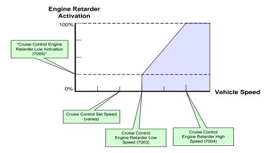
The following programmable parameters, shown in the graph, are customer adjustable. Default settings are used in this example:
