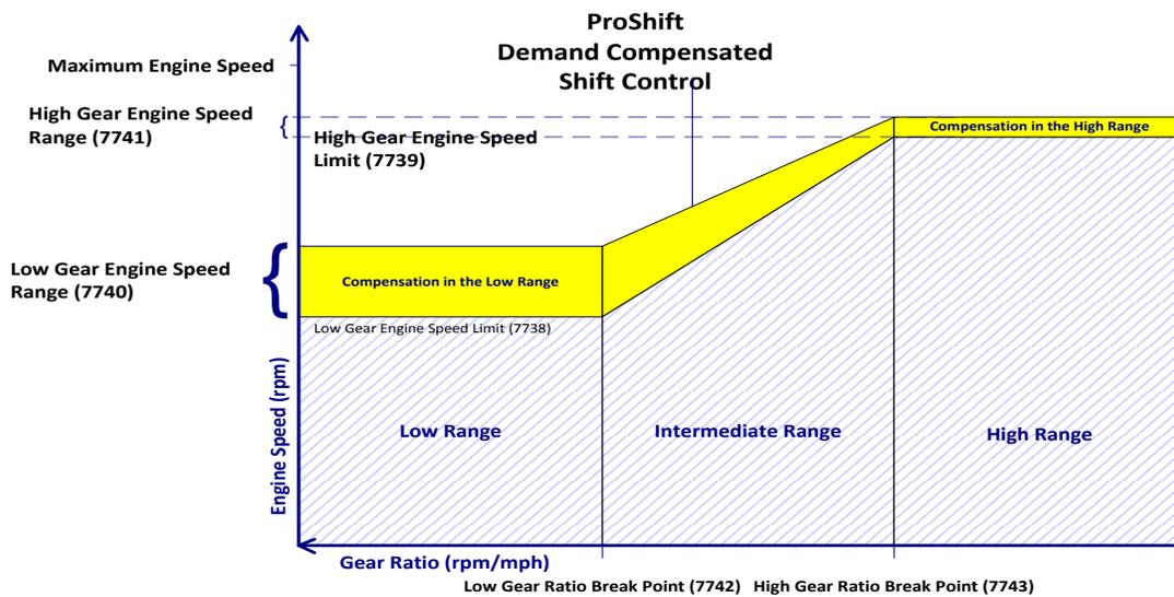
ProShift consists of 3 gear regions: a high gear region, a low gear region, and an intermediate region. The gear ratio break point parameter settings determine what range the gears fall within.
