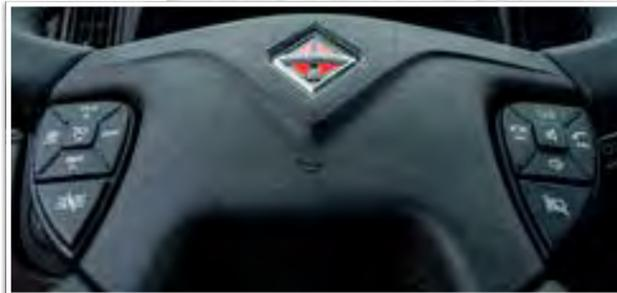
Laser-etched steering wheel controls
