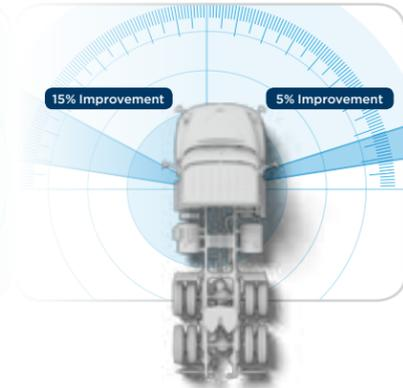
The shaded areas represent how indirect visibility has been optimized by reshaping the doors and side windows, and repositioning the cab mirrors so drivers turn their heads 15% less on the driver side and 5% less on the passenger side. This increased visibility reduces driver stress and neck strain to enhance productivity.
