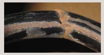
A broken power spring is the leading cause of spring brake failure.
