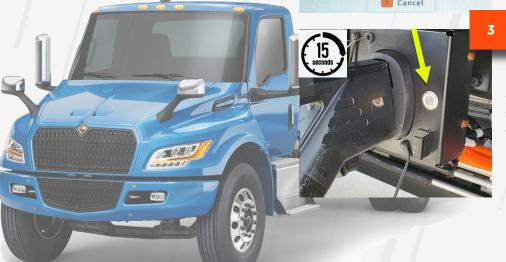
Wait 15 seconds and press the charge interface button a second time.
