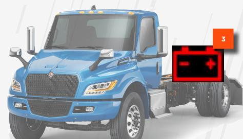
If the 12 volt battery system has low voltage, the red battery indicator will show on the instrument cluster. If this indicator is present, the vehicle will not go into "High Voltage Ready" mode and the vehicle will not be able to start.
