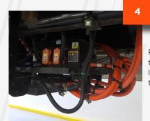
Please pay special attention to HV cables and shielding located towards the rear of the vehicle.
