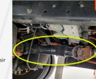
Use a paint marker to record propeller shaft mating positions at the drive motor and rear axle. ELECTRIC
