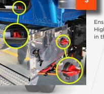
Ensure Low Voltage and High Voltage switches are in the "OFF" position.
