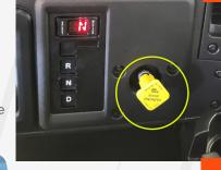
Ensure the parking brake is applied before working under the vehicle.
