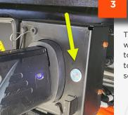
The charge interface button will then illuminate **BLUE** to indicate the charger to vehicle connection is secure.
