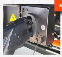
Unplug charging cord by pressing the release button on top of the charging handle.
