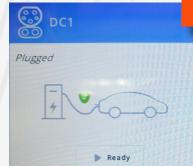
Click READY button on the charger screen to start charging process for vehicle #2.
